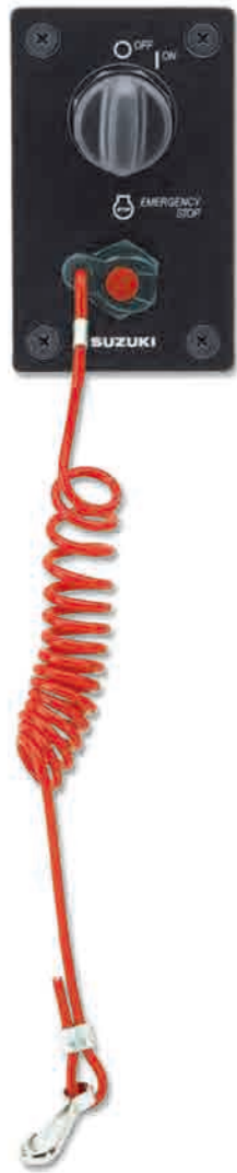
37100-98J04-000 single ignition with Emergency-stop switch
