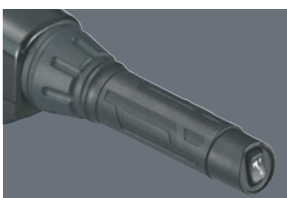
Power trim & tilt switch and throttle grip friction adjuster
